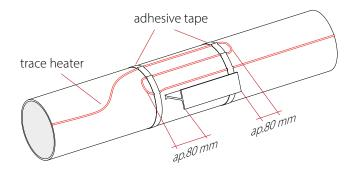
In areas of pipe supports, trace heaters must be laid in a looped manner in order to be able to provide sufficient power at this point.
