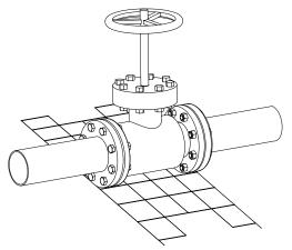
• Cut the wire guard to size so that it fits exactly
