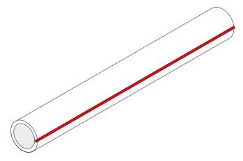
Normally the trace heater is laid streched out along the pipe. Lay trace heaters in a spiral pattern only if the projects planning explicity calls for it.
