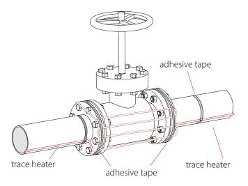
• In areas with large pipe diameters, trace heaters must be laid in a loop.
