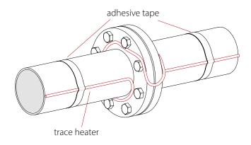
When laying a trace heater around a flange connection, it
