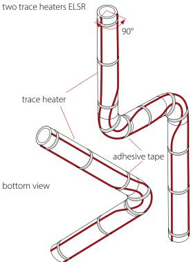
When laying a trace heater around a pipe bend, the trace heater must be laid on the outside of the pipe bend. If it is laid on the inside, the flow medium may be deposited in the pipe due to the lower heat input to the pipe.
