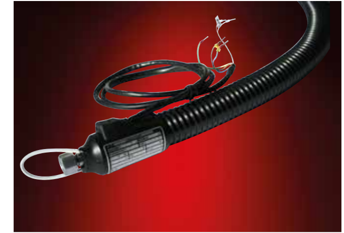
ELH/mdw-200 °C-DN10 Heated pressure hose with excess heated cable length For heating the connection fitting. Application: Plant engineering / transporting oil and grease for a coating system
