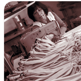
Handicraft: the eltherm-manufactured heating cables are sewed together with the according insulation custom-fit to the backing fabric of the heating jackets and mats.
